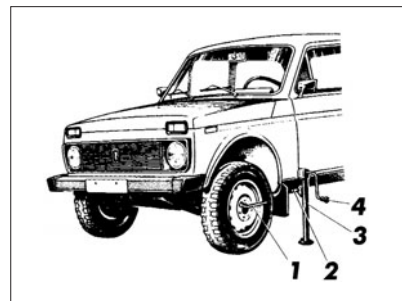
Fig. 42. Lifting the car when replacing wheels
